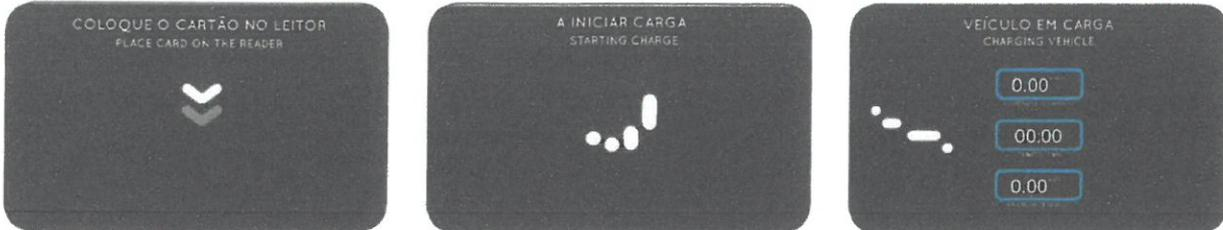
TFT screen display with intuitive menu-based interface permits the user to have an immediate graphic perception of the charging process. User access is validated by RFID card. Access password introduction and navigation through the application is done by using capacitive numeric keypad.
